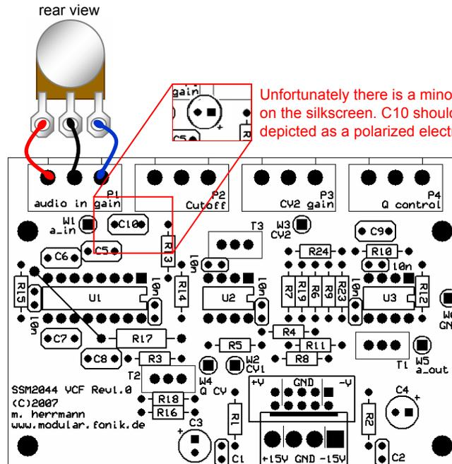
There are 6 decoupling capacitors on the layout not mentioned in the schematic. They are labeled 10n.
