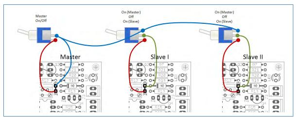
On the 1<sup>st</sup> module (master) the **red** wire connects the clock signal to the Master On/Off switch. From there the clock signal is routed to the master modules comparator section, and to the slave modules On/Off/On switches (**blue** wire). The On/Off/On switches of the salve modules connect either the master clock signal (**blue** wires) or the slave clock signal (**red** wires) to the comparators (**green** wires).
