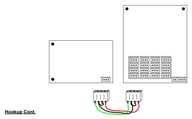
Be sure to connect right most pin to positive. The center two pins to ground and the left most pin to negative.
