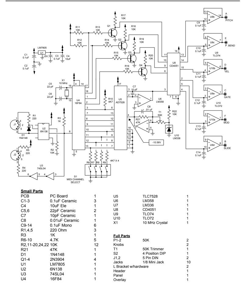
The PIC loads the correct number into the DAC digital to analog converter U5 to generate a voltage that corresponds to the midi message received. Then selects which output is active by strobing the demux U8's select pins through the Q1-Q4 inverterbuffers. When one of the outputs goes high the voltage is sampled and held by capacitors C9-C14 until it is refreshed. U6a is the DAC output amp and U6b is the DAC voltage reference amplifier.
