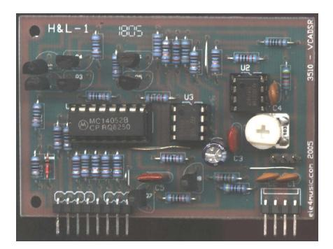
When the gate is removed. Q7 turns off. Q8 turns off and sets the 555s reset pin low.
