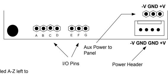
The I/O pins are labeled A-Z left to right. The power header can be a friction lock type to match the power supply or standard pc-board headers.
