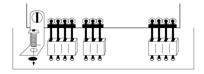
90 degree headers allows you to use the boards on a carrier or mother board. Mix and match to build the synth you want. (Requires a slightly longer L-bracket)
